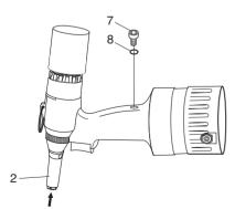
• Bend the riveting tool carefully towards the front at an angle, and fix e.g. inside a vice (like illustrated in the diagram).
