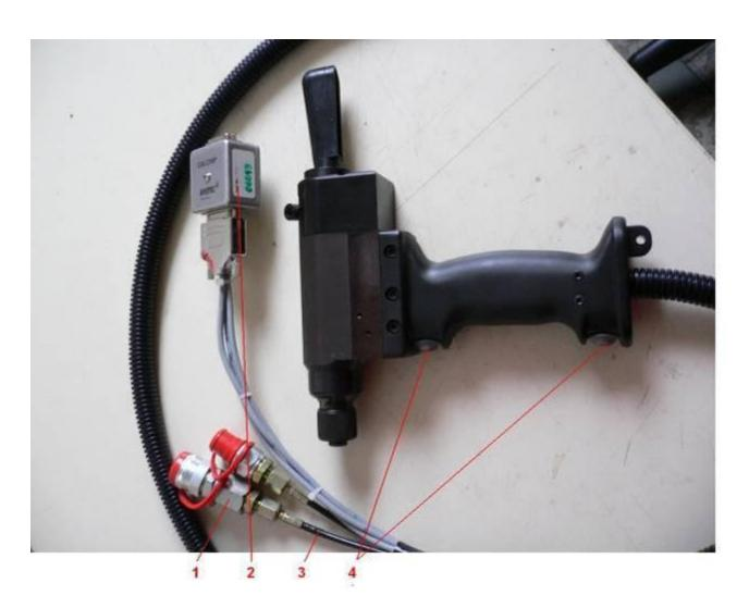
To the riveting head, it is possible to mount various types of riveting nozzles for various types of rivets. The limiting factor when choosing is the opening diameter in the hydraulic piston of the riveting head, the dimension of the connecting threads and openings, and the force needed for rivet tearing off. In case of any doubt, it is necessary to address the authorised service or the manufacturer.
