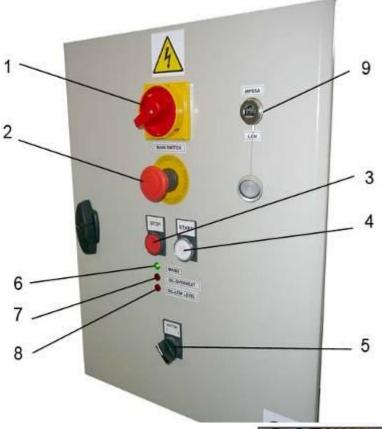
Power control light (6), main switch (1), central STOP (2), aggregate start (4), aggregate stop (3), button switch (5) – serves for activation of the corresponding button at the riveting head, oil overheating control lamp (7), low oil level and filter fouling control lamp (8), LAN (9).
