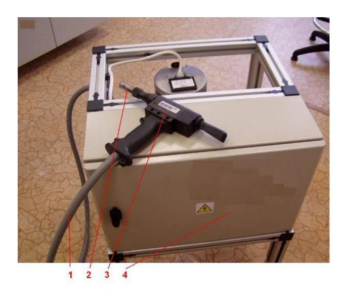
The riveting nozzle that is fastened to the riveting head, they must correspond to the rivet to be riveted. The connecting hose serves for connecting the riveting head with the drive unit and at the same time allow for increasing the action radius of the operator. The drive unit serves as a source of pressure oil for riveting head drive and at the same time it secures control, checking, and evaluation of the entire riveting process.
