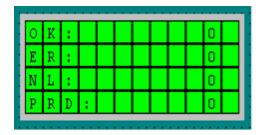
OK riveting counter NOK riveting counter Reset impulses counter Idle cycles counter
