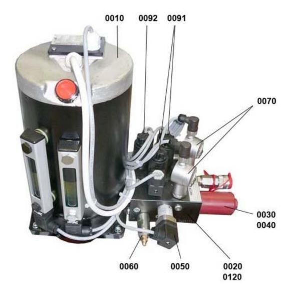
The aggregates may only be operated in a short-term operation S2 or an interrupted operation S3 (according to VDE 0530). They are not suitable for permanent loading with the working pressure. Overheating may cause motor burning or plastic part melting. Besides that, there is also the danger of injury! The aggregate contains thermal protection of the motor.
