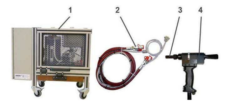
The nose assembly that is fastened to the riveting head, they must correspond to the rivet to be riveted. The connecting hose serves for connecting the riveting head with the drive unit and at the same time allow for increasing the action radius of the operator. The drive unit serves as a source of pressure oil for riveting head drive and at the same time it secures control, checking, and evaluation of the entire riveting process.
