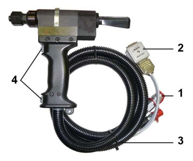
To the riveting head, it is possible to mount various types of nose assemblies for various types of rivets. The limiting factor when choosing is the opening diameter in the hydraulic piston of the riveting head, the dimension of the connecting threads and openings, and the force needed for rivet tearing off. In case of any doubt, it is necessary to address the authorised service or the manufacturer.
